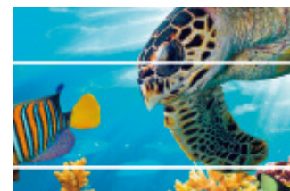
Gap/White streaks (Excessive feeding amount)
